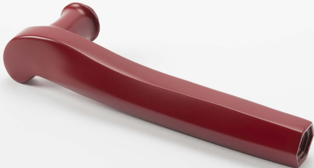
PRISMA BORDEAUX OPACA COD. PROD-PRI.06 MATERIAL-aluminium FINISH-bordeaux painting TECHNIQUE-aluminium casting SIZE-16x3,8x5 cm
